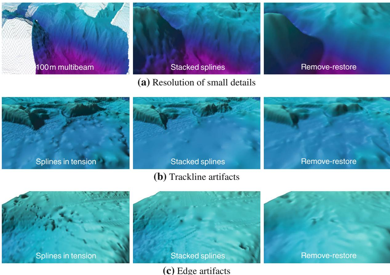
**Fig. 3** In their details, the three compared grids vary significantly. The *stacked splines* grid preserves a lot of small morphological features from the source data, which are lacking in the *remove-restore* results (a). Both the *remove-restore* and the *stacked splines* approach give pleasing results in areas with sparse source data, where *splines in tension* develop distracting track line artifacts (b). With regard to
