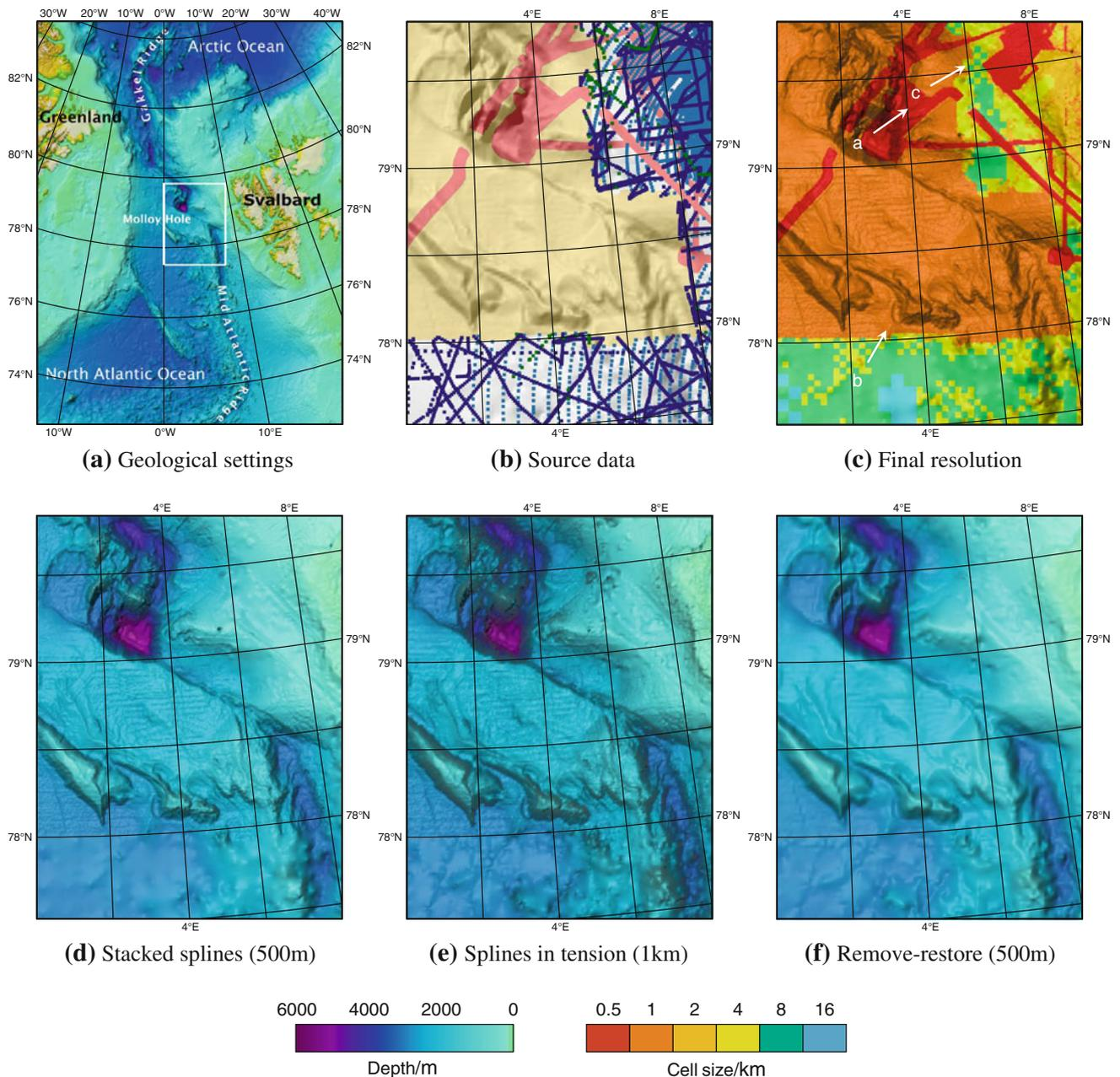
**Fig. 2** Comparison of various spline interpolation based gridding methods, using an identical source data set (b), comprising 100 m and 1 km multibeam grids (red and yellow, respectively), single beam soundings (blue) as well as submarine measurements (green). The results differ in the level of preserved small morphological details, the amount of artifacts at insufficiently constrained places or data set
