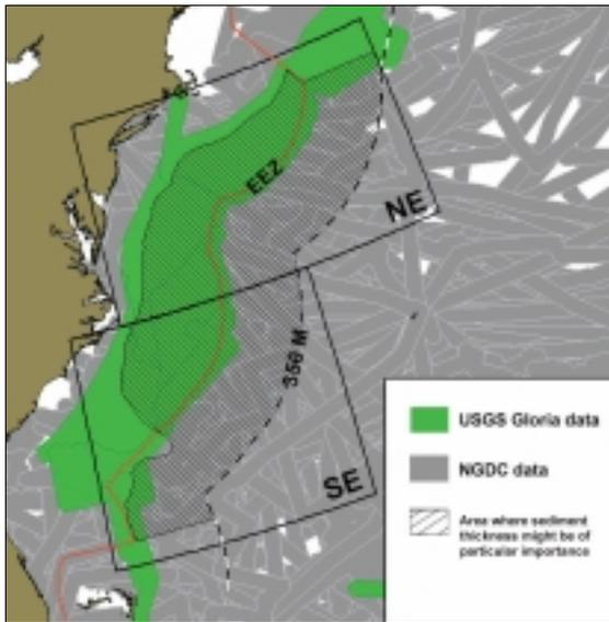
Figure 8: Example showing 15 nautical miles (30 nautical miles wide trackline) buffer zones generated in Geomedia Pro around seismic tracklines from NGDC and the U.S.G.S. Gloria project. This was done to analyse if the line spacing was more than 30 nautical miles
