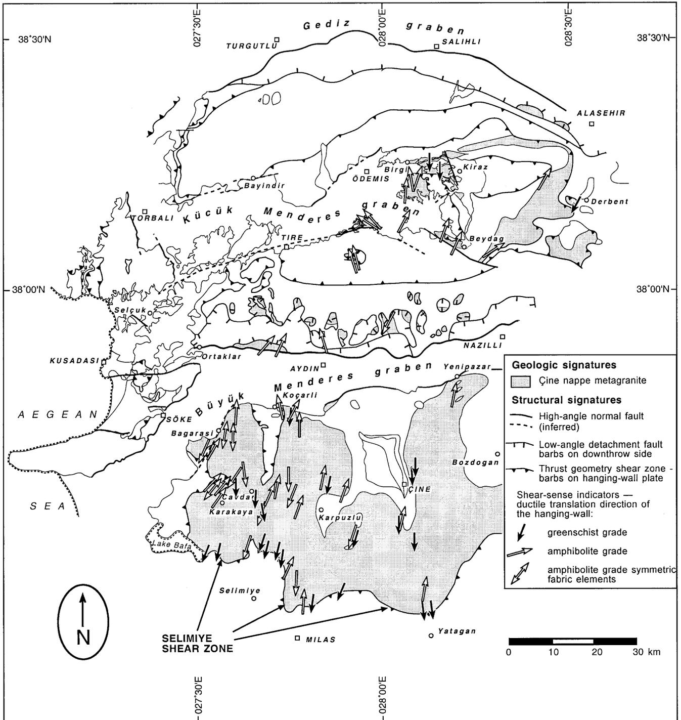
**Fig. 6** Map shows  $D_{PA}$  (white) and  $D_{A3}$  (black) kinematic indicators in the Çine nappe granitoids. Arrows point to movement direction of the hangingwall
