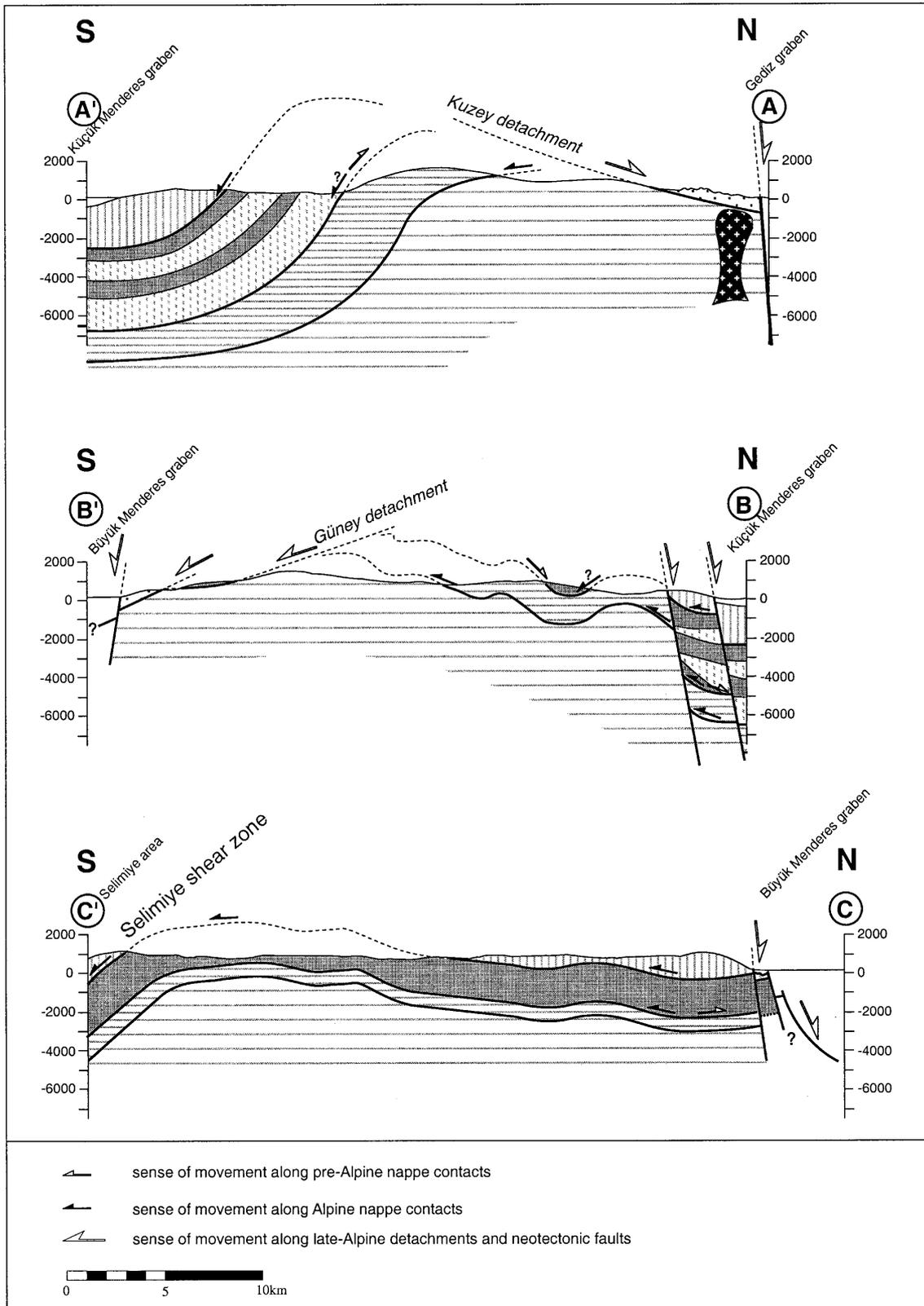
**Fig. 2** Geological cross sections along section lines  $A-A'$ ,  $B-B'$  and  $C-C'$  as illustrated in Fig. 1. Projection of foliation planes and fold axes into the section plane and extrapolation of large-
